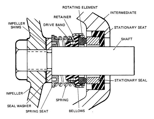
Figure 2. 25271-821 Seal Assembly
